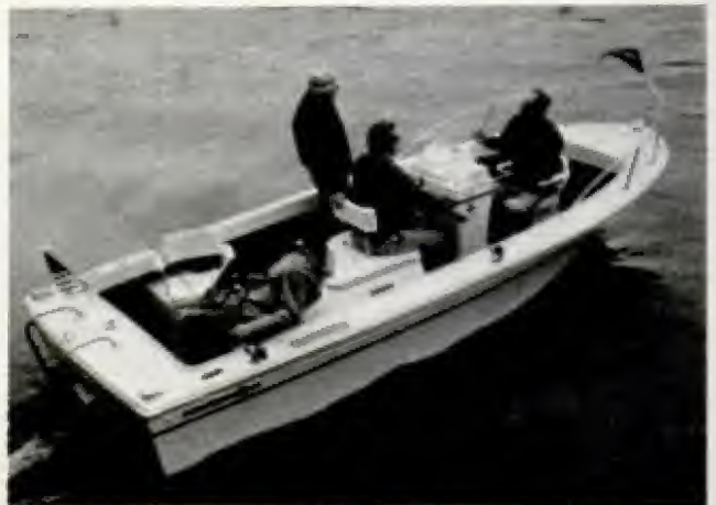
MARINE ALUMINUM is used in a number of "off-shore" models. Above, Chrysler's Fin Runner weighs but 875 pounds, yet can carry 3000 pounds. $1730
